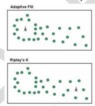
Ripley's K may require use of the minimum distance constraint as nodes of low sampling density will likely be clustered together. Previous versions of SADA simulated the placement of Ripley k values to offset this problem. This approach will be reinstalled into SADA in the near future. In the meantime, we must rely on the minimum distance constraint.
