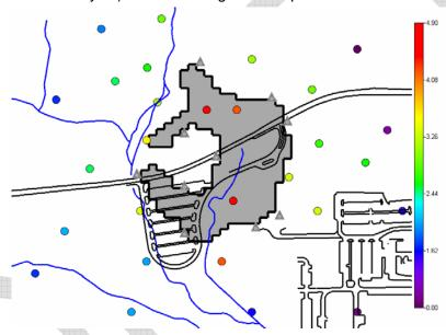
Notice that new sample closely follow the AOC boundary line and space them out rather evenly when the minimum distance constraint has been imposed.
