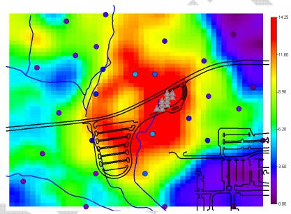
You can see that strict adherence to choosing the highest value nodes results in severe clustering in one local area where several nodes are among the highest. Now recheck the Separate by at least option in the Set sampling parameters step. Press Show The Results once again.
