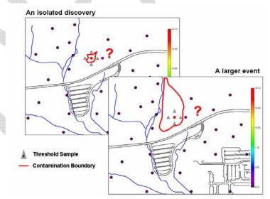
When you execute the threshold design, SADA will ask you for a decision criteria. Those measured values that exceed this criteria will be the target of the sampling design. Normally this decision criteria is a single value typically the screening value (see chapters on performing data screens). However recall that under the General analysis it is possible to specify depth specific decision criteria. In the example that follows we will use a two dimensional (surface)
